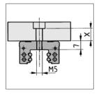
In the case of slide guides with two parallel guide rails, the fastening screws of the slide should be securely attached to the guide carriage, following parallel alignment. The loose screws of the rails should then be tightened in the sequence indicated, by applying the specified tightening torque (refer to the section 'Installing the Guide Rail').
