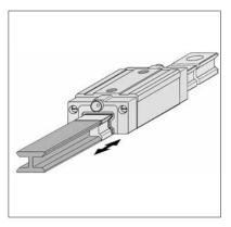
Carefully push the carriage once along the entire length of the guide rail and check the resistance to movement, particularly as the carriage passes over the plastic plugs (reset them if necessary). Any perceptible friction is principally attributable to the fact that the seals have not yet bedded in; this friction will diminish when the flexible elements have settled and adjusted to the rail.
